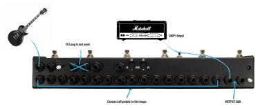
In this configuration, all pedals are IN FRONT of the amp as we are not using the FX LOOP module.
