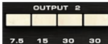
**OUTPUT 2 delay buttons:** This switch group controls the delay of the second output. It is operative regardless of the setting of the DELAY ONLY switch. Delay 2 is fed from the sum of the input to the H910 and the main feedback path. Delay 2's input is connected before the input to the pitch shifter
