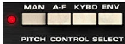
**PITCH CONTROL SELECT switch group and LED indicator:** When the PITCH CONTROL mode is activated, the LED INDICATOR immediately to the left of the PITCH CONTROL SELECT switch group becomes illuminated, and the four switches assume control of the pitch change function.
