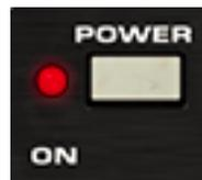
**POWER button and LED indicator:** The power button functions as a bypass switch. When the POWER button is depressed the H910 plug-in is active. Otherwise the H910 plug-in is inactive and if the DSP can be unloaded it will be.
