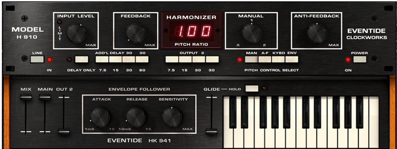
The H910 user interface consists of two parts. The top half of the interface is the front panel of the original H910 2U rack mount unit. All controls function in the same way as the original. The bottom half of the interface enables features originally available through external connections or options.
