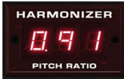
**PITCH RATIO readout:** An LED readout gives the numerical pitch ratio of the Harmonizer. As this is a true digital readout, it is not subject to miscalibration and may be used as a precise reference.
